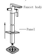
7.Fix flange with locking screw to faucet body firmly.
