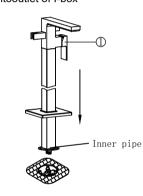
9.connect flange and I-box with locking screw, tighten with allen key. Close panel to the floor.
